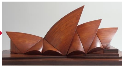
Arup wind tunnel model
